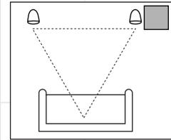
The center channel speaker should be placed slightly behind the front left and right speakers, and no more than two feet above or below the tweeters of the left and right speakers. It is often convenient to set the center speaker on top of the television set, as shown in the drawing. Use the supplied support leg to aim it toward the listener by screwing the leg in to angle the speaker up, or unscrewing the leg slightly to angle the speaker down.
