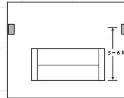
The two surround speakers should be placed slightly behind the listening position and, ideally, should face each other and be at a level higher than the listeners' ears. If that is not possible, they may be placed on a wall behind the listening position, facing forward. The surround speakers should not call attention to themselves. Experiment with their placement until you hear a diffuse, ambient sound accompanying the main-program material heard in the front speakers.
