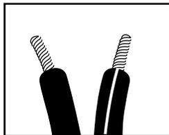
Separate and strip the ends of the speaker wire as shown. Speakers and electronics terminals have corresponding (+) and (-) terminals.
